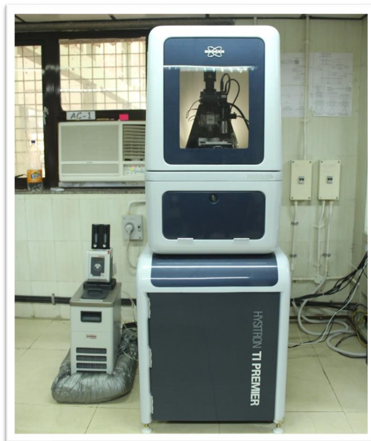
Figure 2.14: Nanoindentation setup used to evaluate the mechanical properties of the deposited films
