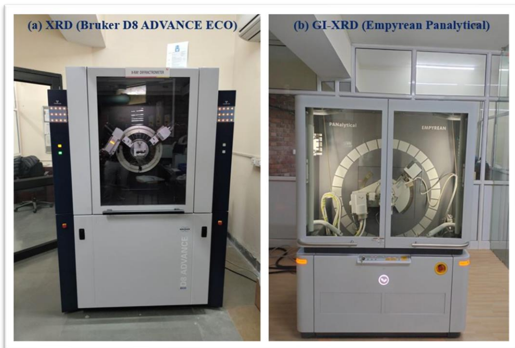
Figure 2.7: X-ray diffraction (a) XRD (Bruker D8 ADVANCE ECO) (b) GI-XRD (Empyrean Panalytical)
