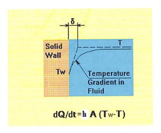
Fig: 1.1 Conduction through a wall
