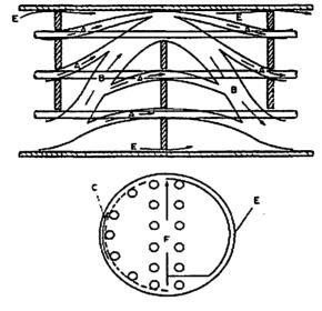
Shell-side leakage and by-pass paths
