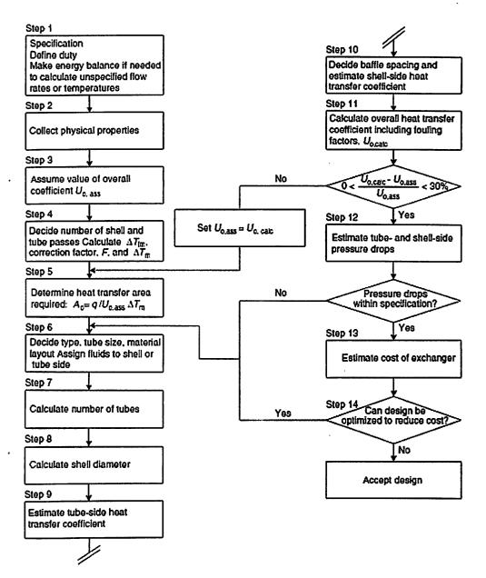
Fig: 2.1 Algorithm for designing
