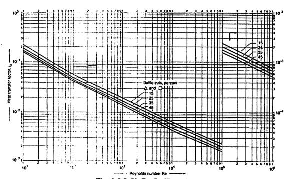
Fig: 2.5 J<sub>h</sub> Vs Re (baffle cut)
