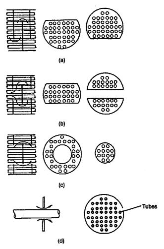
Types of baffle used in shell and tube heat exchangers. (a) Segmental (b) Segmental and strip
