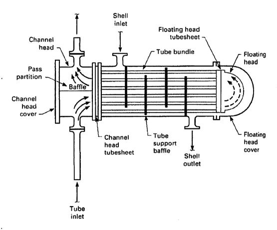
Fig: 1.4 Shell and tube heat exchanger
