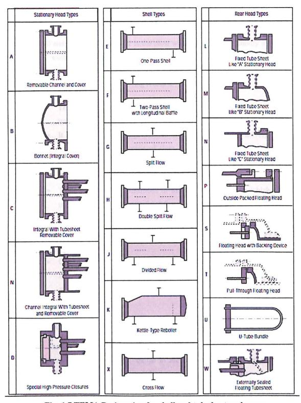
Fig: 1.7 TEMA Designation for shell and tube heat exchanger
