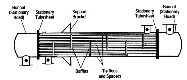
Fig 1.5 Fixed tube sheet
