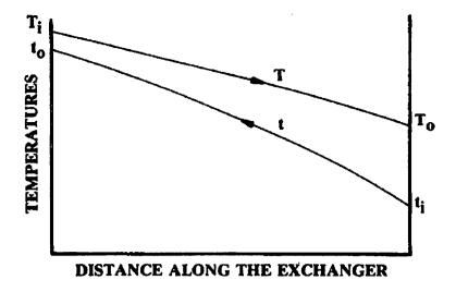
Fig: 1.3 LMTD for counter current
