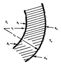
Cross-section of Fluid-to-Fluid Heat Transfer
