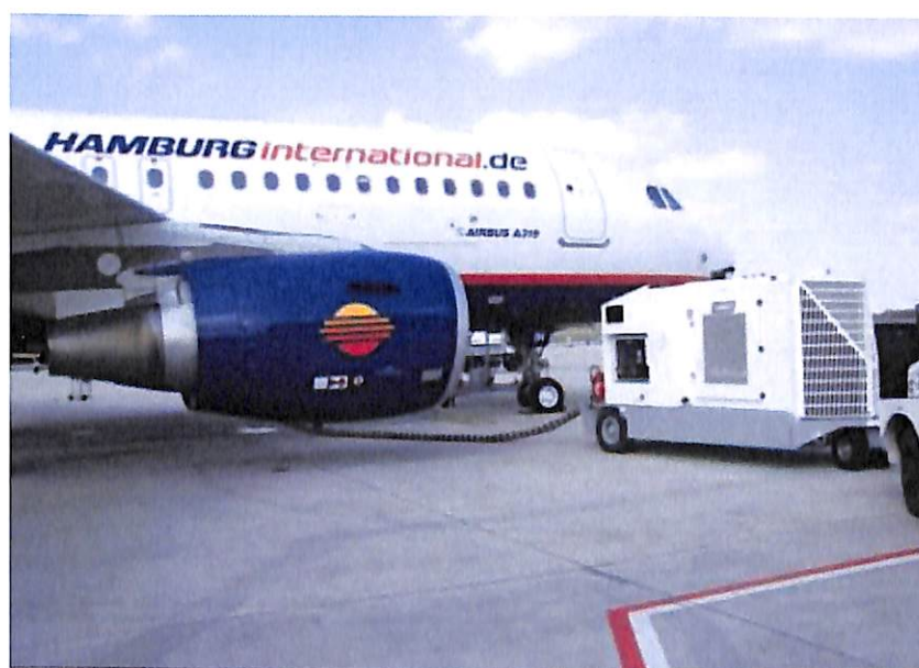
Figure: Air Start Unit (ASU)
