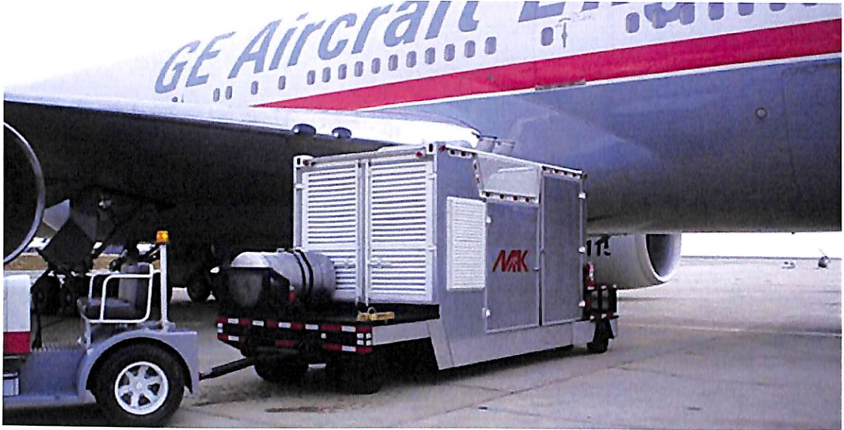
Figure: Ground Power Unit (GPU)
