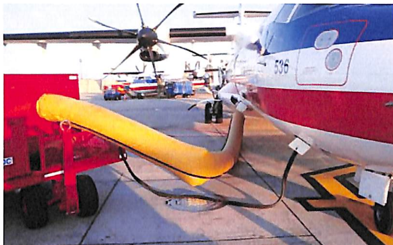
Figure: Air Conditioner Unit (ACU)
