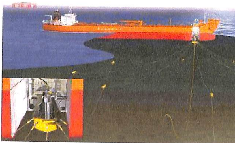
Figure 8.5: Illustration of APL Submerged Turret Loading System
