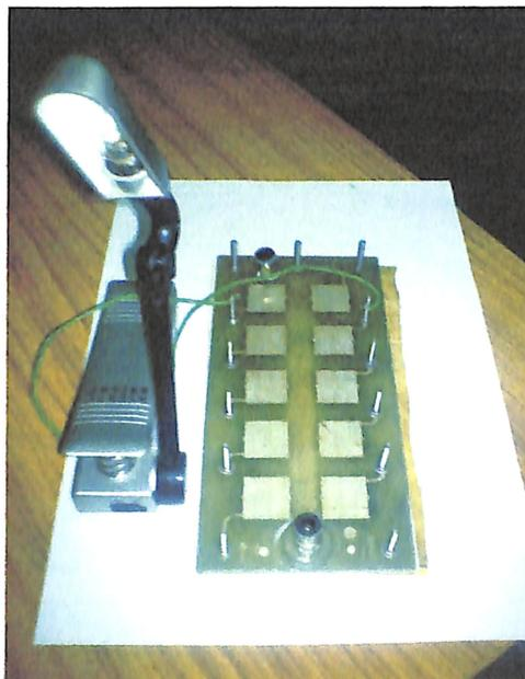
**Figure 14 : Photograph of fuel cell with table lamp**
