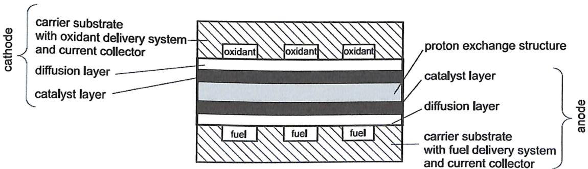
**Figure 4: Basic components of a typical micro fuel cell**
