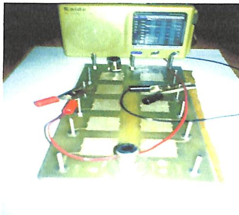
**Figure 12: Photograph of small fuel cell with transistor radio**
