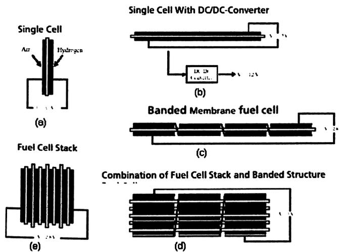
**Figure 6: Construction principles of PEMFC**
