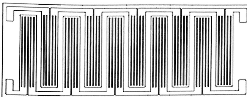
**Figure 8 : Interlaced Flow Channels with Alternating Fuel/Oxidant Chambers**
