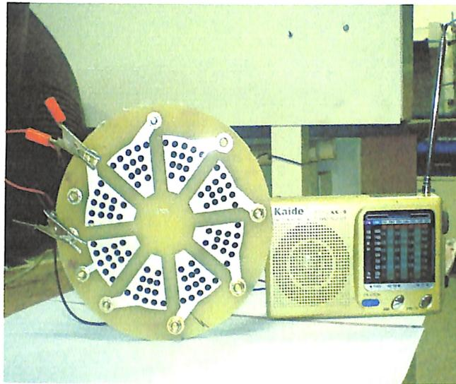
**Figure 21 : Transistor Radio running on a circular fuel cell**
