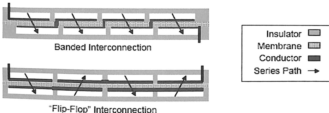
**Figure 7 : Multi-cell interconnection with Flip-Flop configuration**
