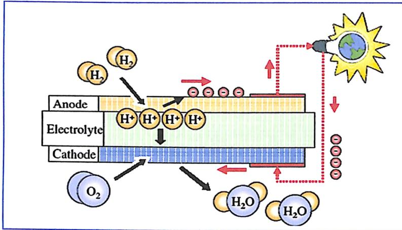
**Figure 1: Working of a Fuel Cell**
