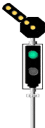
Junction Route Indicator, choosing one among two routes. The indication is for the tracks to the left
