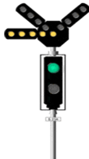
Junction Route Indicator, choosing one among four routes. The indication is for the tracks to the left
