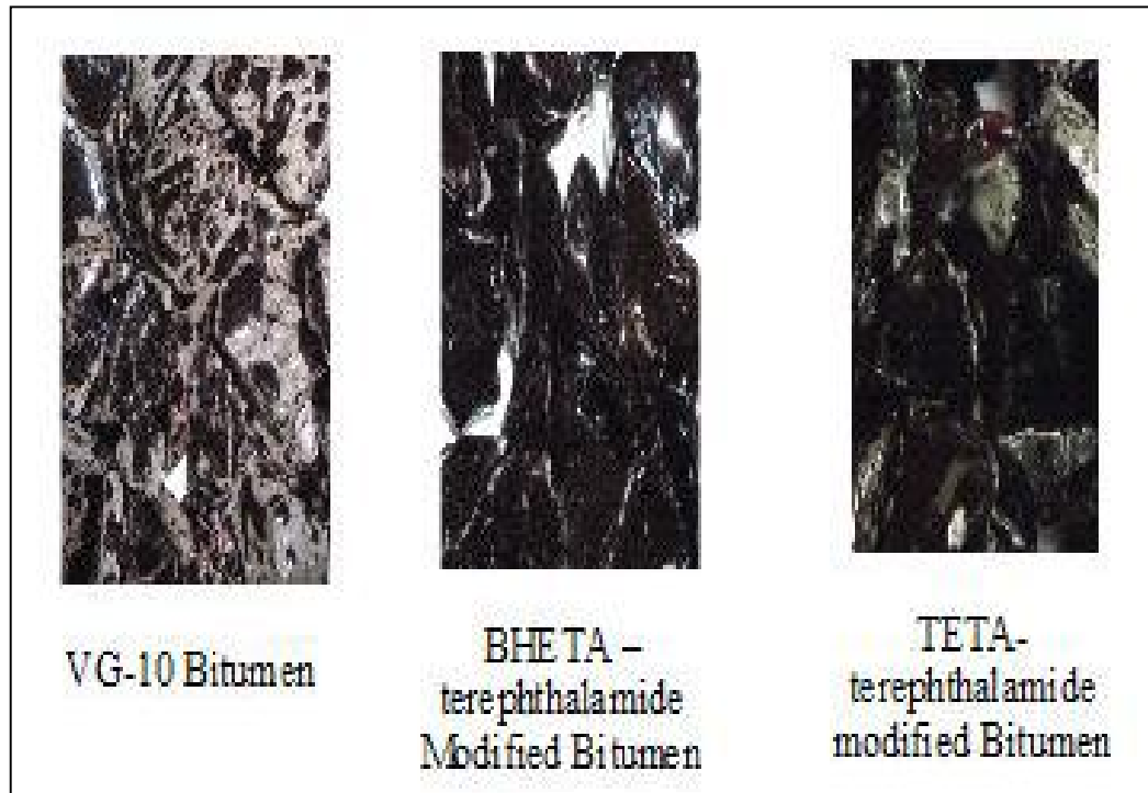
Fig.3.3 Hot water stripping test (ASTM D 3625-96 (Reapproved 2005))
