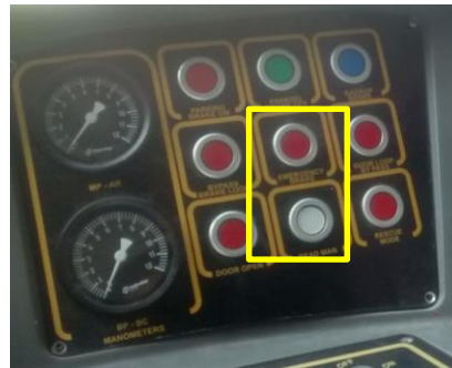
Figure 20: Dead Man and Emergency Brake Indicators
