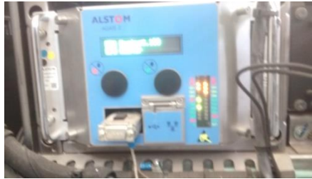
Figure 8: Main Processing Unit (MPU)
