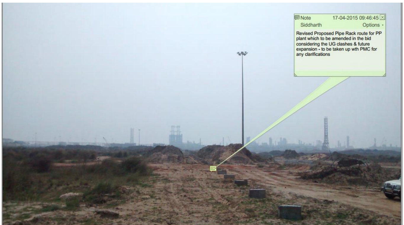
Figure 5.2: Revised Proposed Pipe Rack Route
