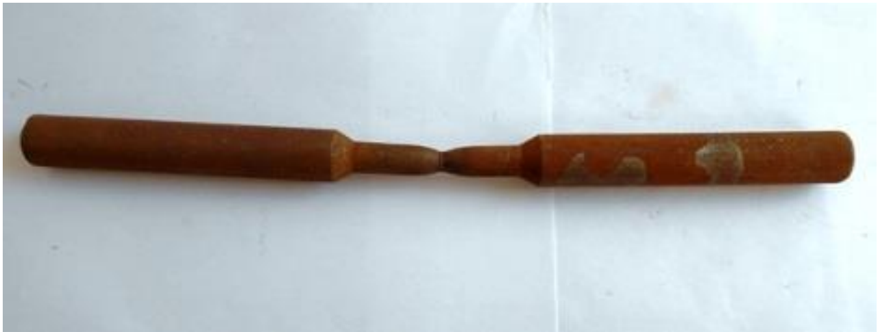
Fig 8: Bare Corroded UTM Test Specimen
