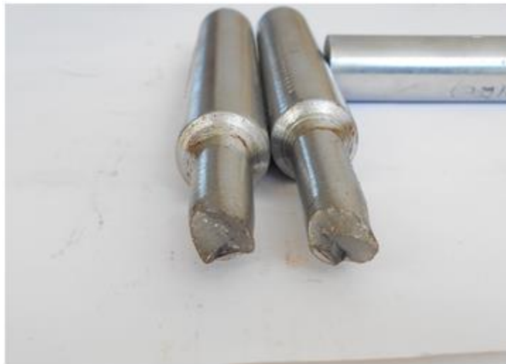
Fig 10: Corroded Coated UTM Specimen
