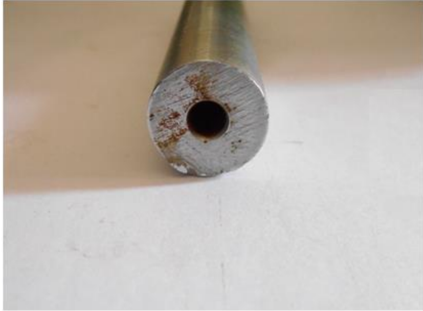
Fig 9: Corrosion on Coated Specimen
