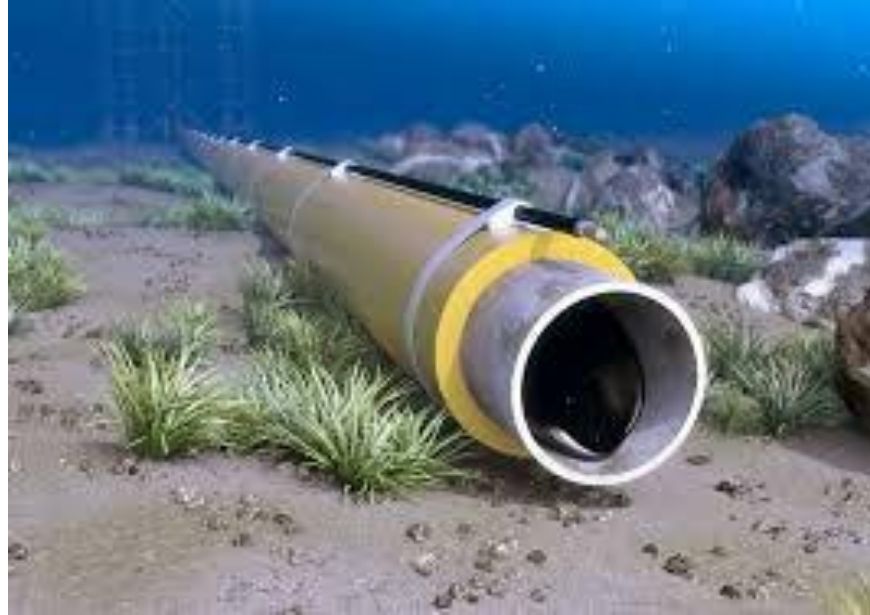
Figure 1: The 9000 kW system used to heat 43 km long subsea production pipeline between Lianzi Field and Benguela Belize Lobitio Tomboco (BBLT) (Source: www.techrelease.com )
