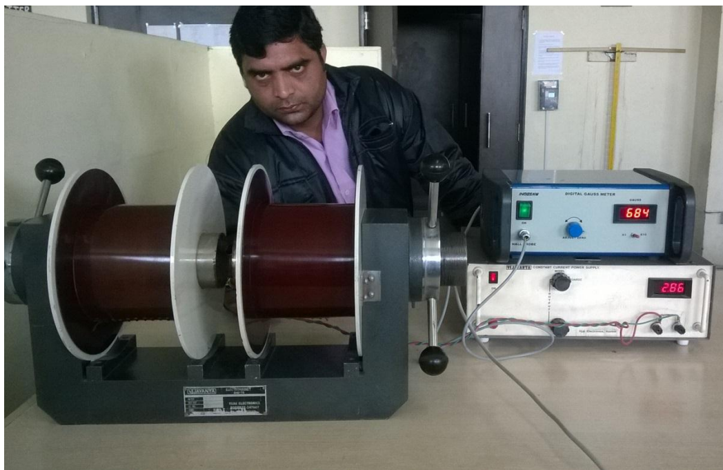
Figure 16: Hall Effect Equipment and Accessories (684 x10 Gauss reading at 2.86 Ampere Current with 1.25 Inch Air Gap Between the two poles of Electromagnet)
