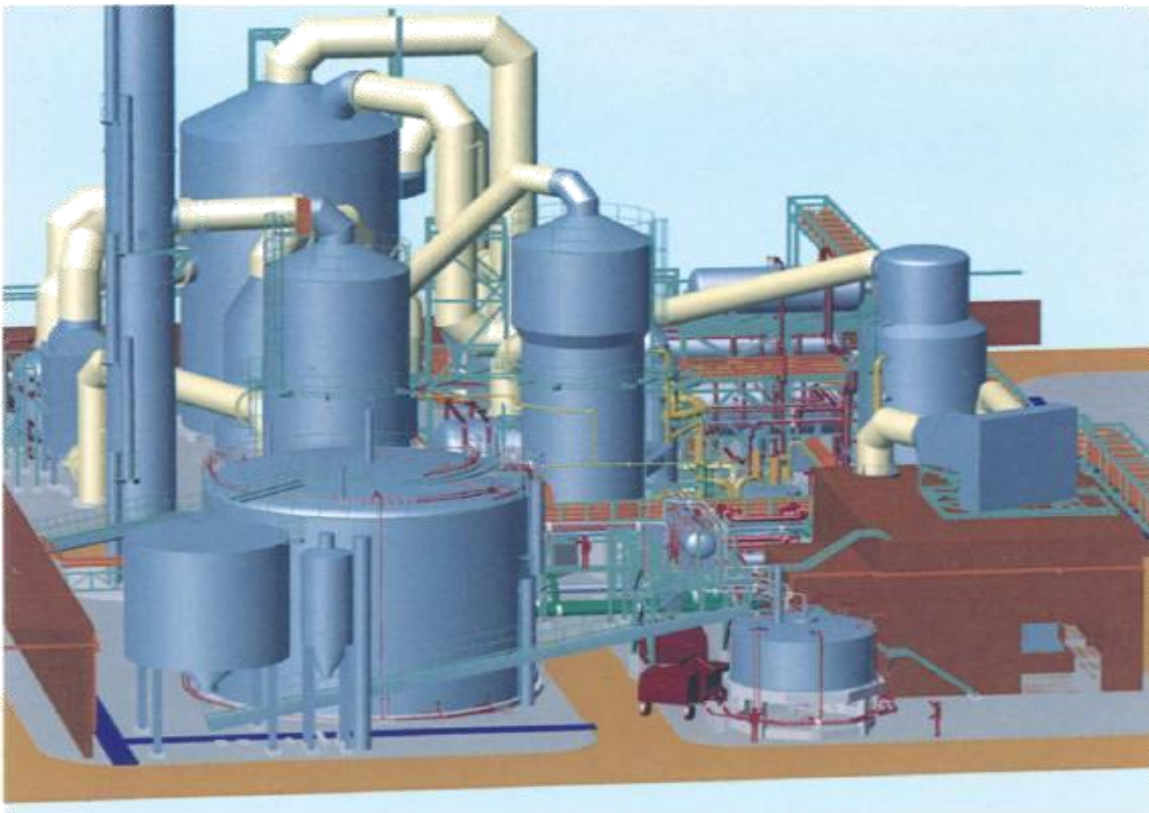
Fig. 2.3. Schematic of sulfur burning sulfuric acid plant, courtesy Outokumpu OYJ www.outokumpu.com . The main components are the catalytic \text{SO}_2 + \frac{1}{2}\text{O}_2 \rightarrow \text{SO}_3 'converter' (tall, back), twin \text{H}_2\text{SO}_4 making ('absorption') towers (middle distance) and large molten sulfur storage tank (front). The combustion air filter and air dehydration ('drying') tower are on the right. The sulfur burning furnace is hidden behind. Catalytic converters are typically 12 m diameter.
