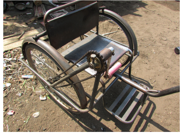
All surfaces including the seat back rest are in metal which get hot during summers and cold during winters
