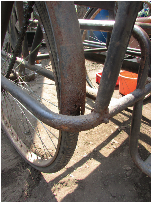
Metal parts rust due to exposure to environmental conditions
