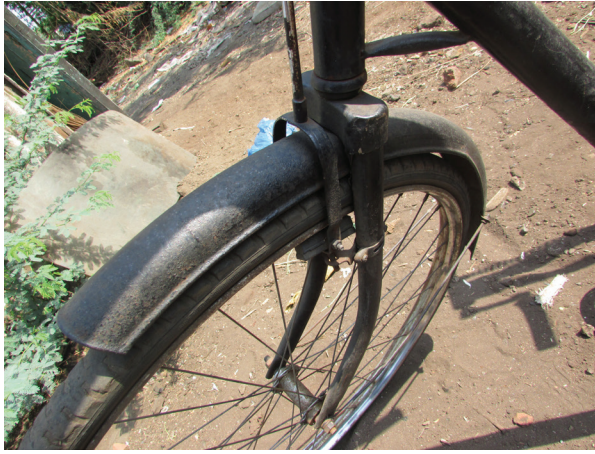
Calliper brakes only on front wheel
