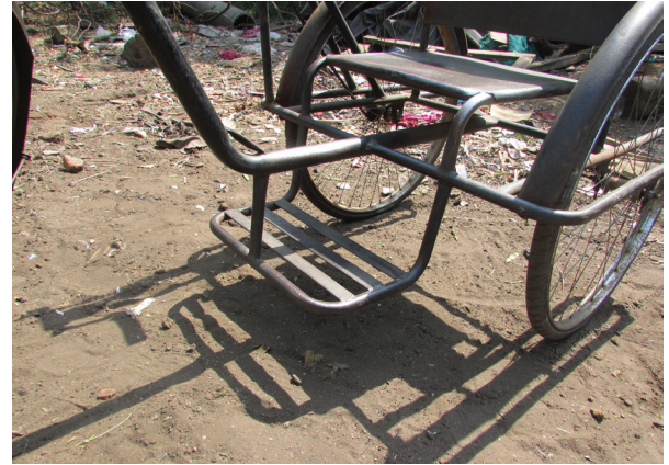
Footrest in metal gets hot as the user wears no shoes
