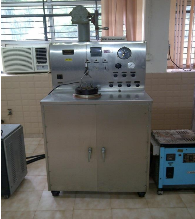
Fig No. 8 HPHT CURING CHAMBER
