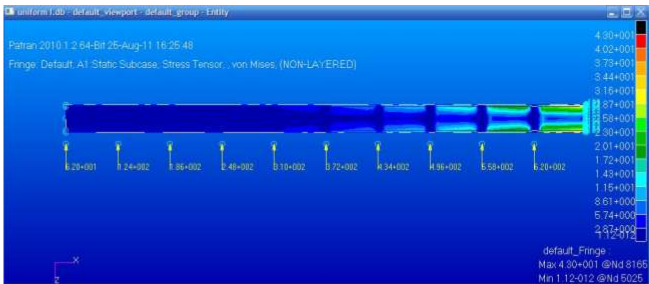
Fig. 4.10 Stress results for Uniform I-section Spar beam.
