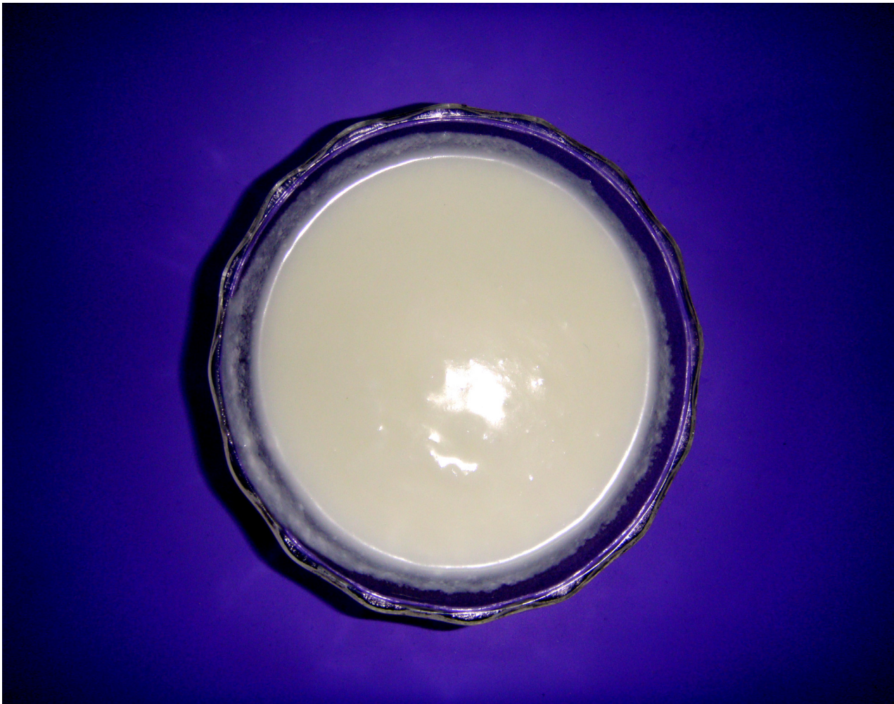
Figure 3.5 Chloride free hydrous zirconia before vacuum filtration.
