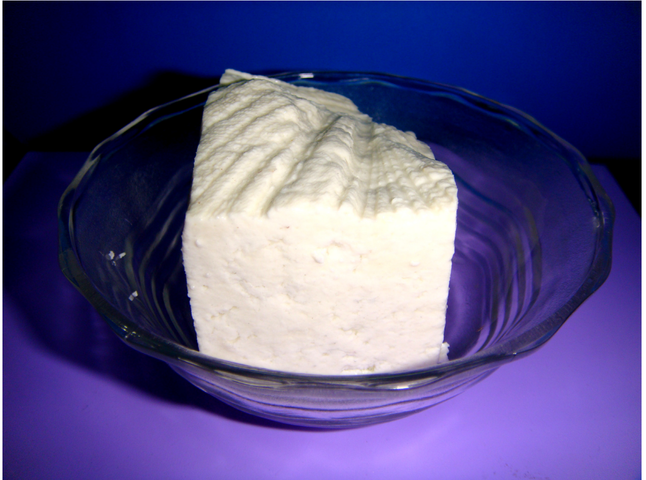
Figure 3.6 Chloride free hydrous zirconia after vacuum filtration.
