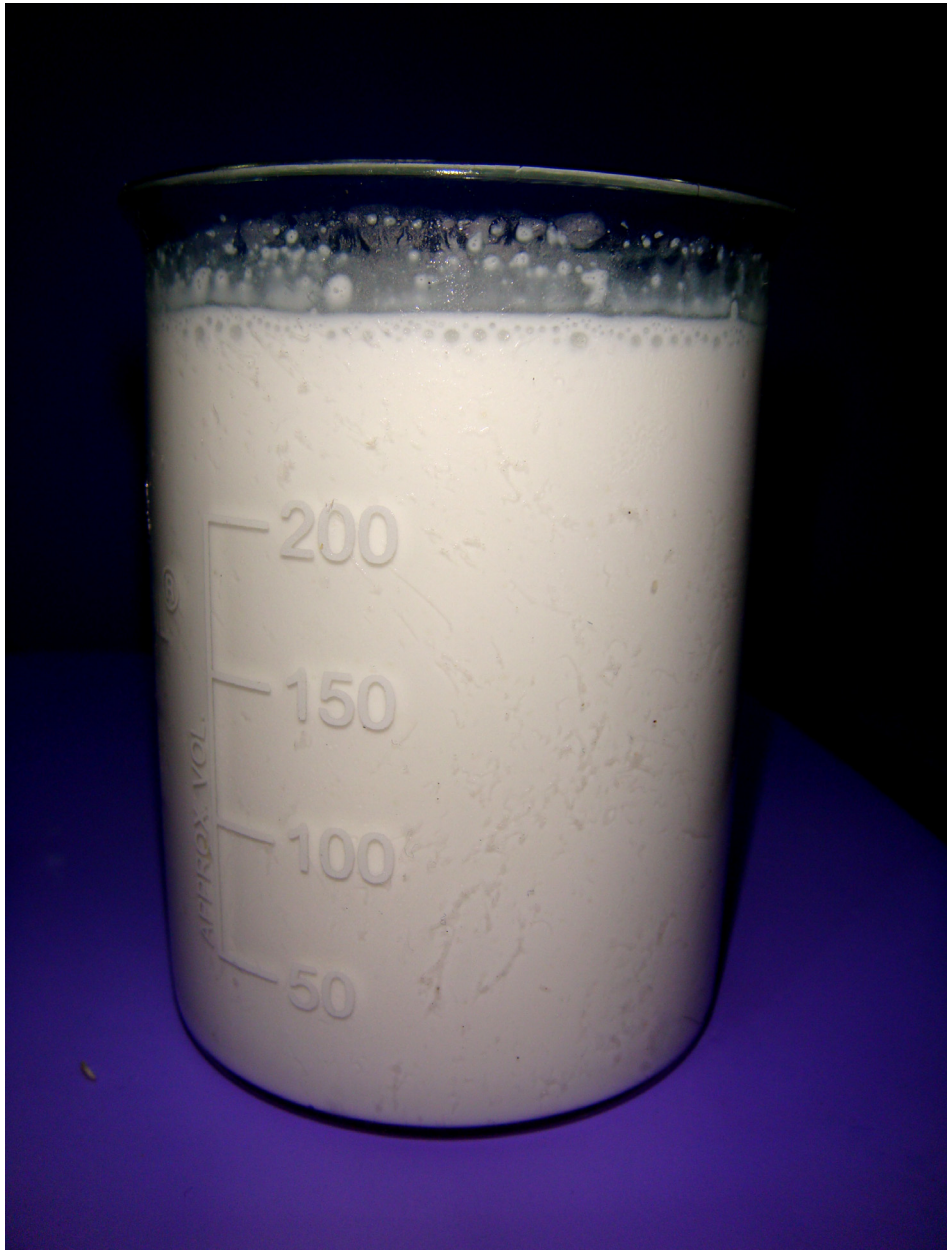
Figure 3.3 Hydrous zirconia after precipitation for 4 hour.
