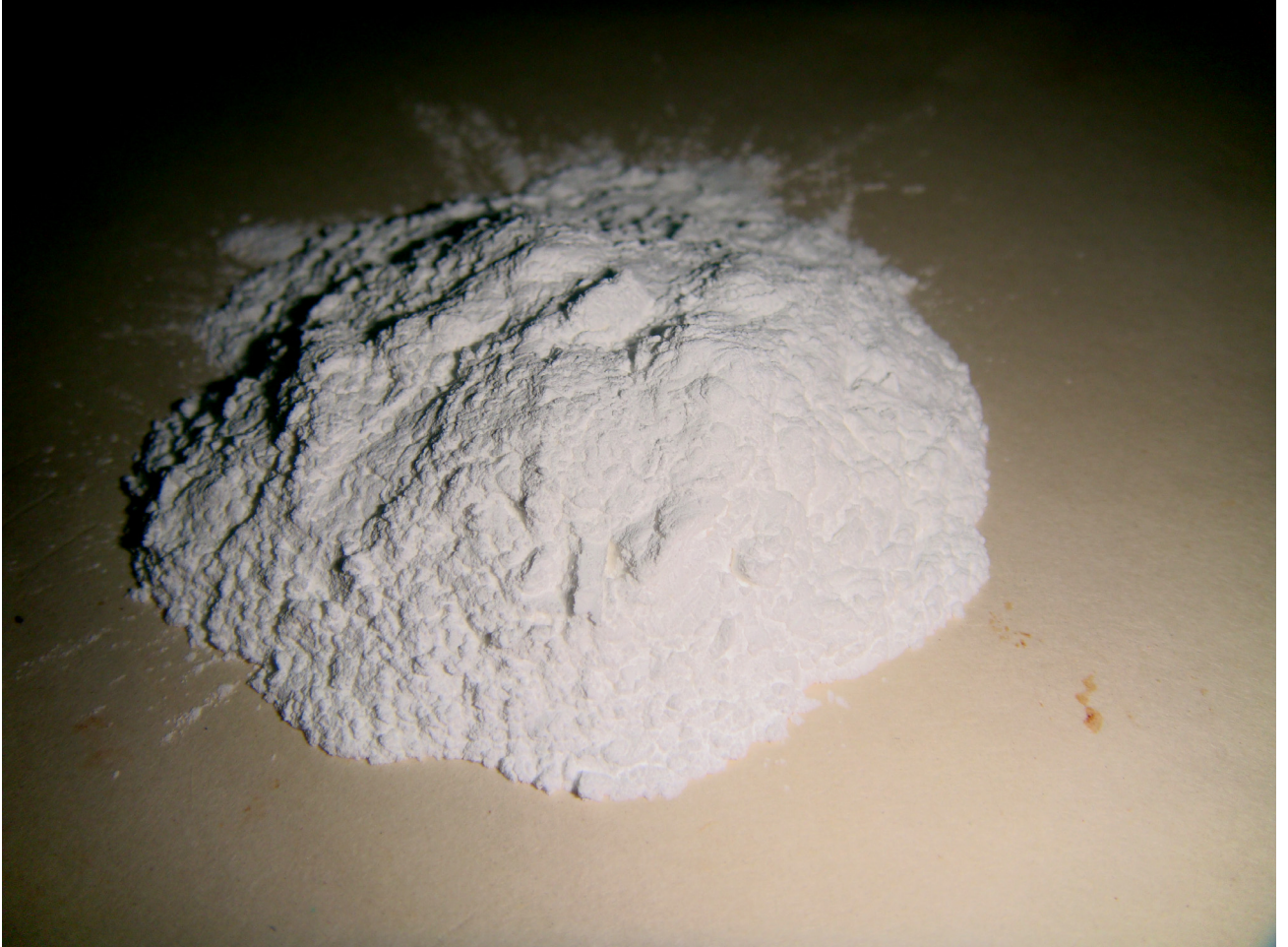
Figure 3.9 Zirconia powder after calcination at 893 K, crushing and sieving to 50 micron.
