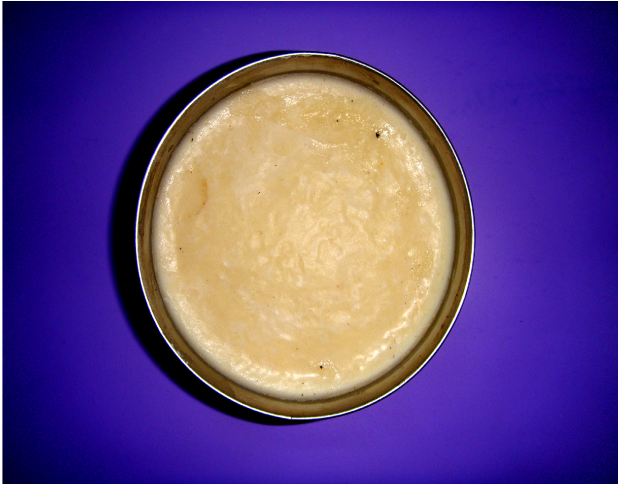
Figure 3.4 Hydrous zirconia after refluxing-aging at 353 K for 6 h.
