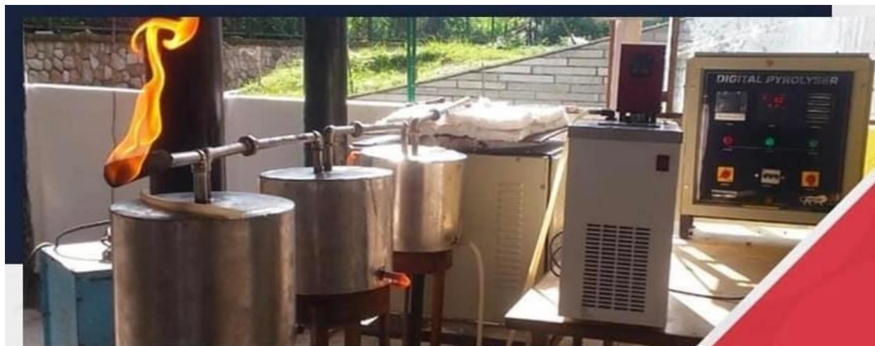
Figure 4.3 Reactor in series with condensation for the pyrolysis-based production of hydrocarbon fuel.
