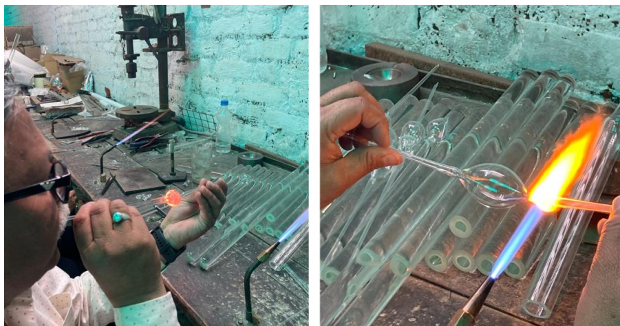
Fig. 3.7 Blowing air to create desire shape
