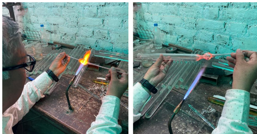
Fig. 3.6 Heating till it softens to blow air
