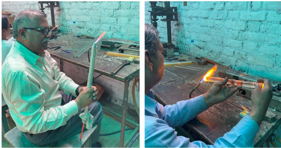
Fig. 3.5 Cleaning and heating the glass pipe
