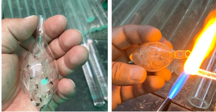
Fig. 3.9 Inserted natural material in the glass and proceeded to close the opening
