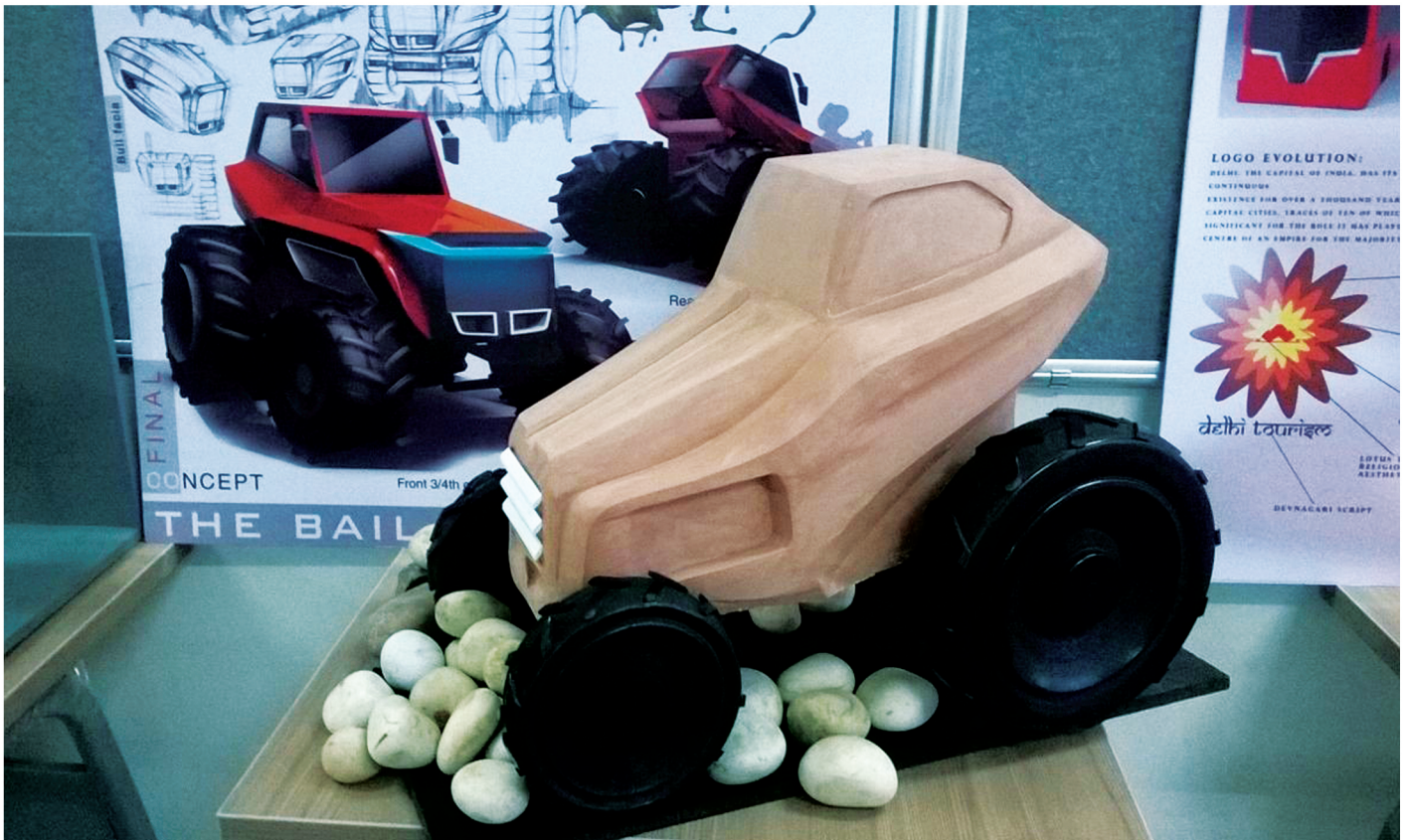
Display model of tractor in clay to scale 1:5
