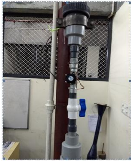
Figure 4.7: Prototype with the Turbine for Testing
