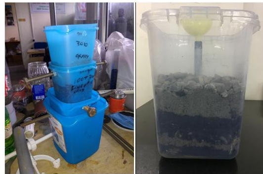
Figure 4.3: Different stages of lab testing to check for filtration unit and mechanism
