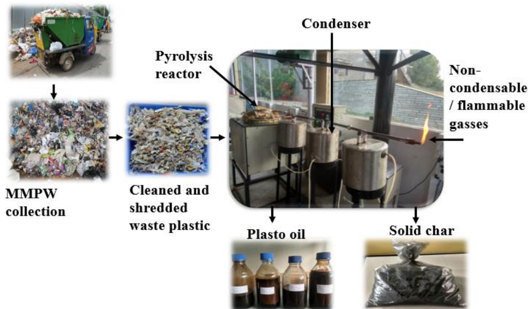
Figure 3.10: Conventional pyrolysis process of the MMPW
