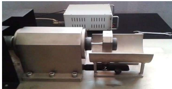
Fig. 4.14. Rotating beam fatigue machine used For testing the specimen
