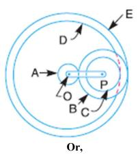
A reverted epicyclic gear train for a hoist block is shown in Fig. The arm E is keyed to the same shaft as the load drum and the wheel A is keyed to a second shaft which carries a chain wheel, the chain being operated by hand. The two shafts have common axis but can rotate independently. The wheels B and C are compound and rotate together on a pin carried at the end of arm E. The wheel D has internal teeth and is fixed to the outer casing of the block so that it does not rotate.
