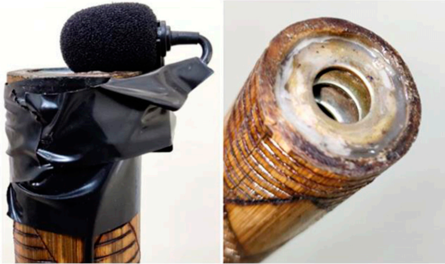
Figure 2. Arrangement of the microphone on top of the flute.
