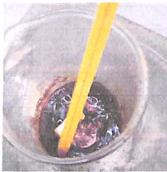
Fig 9: Gel Formation of Fe-Co
