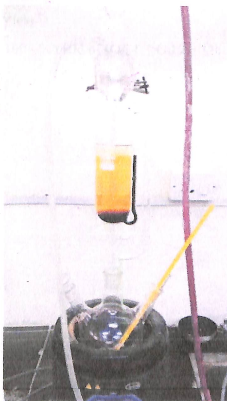
Fig 20: -Extracting Oil 3 from solids using acetone in Soxhlet Apparatus
