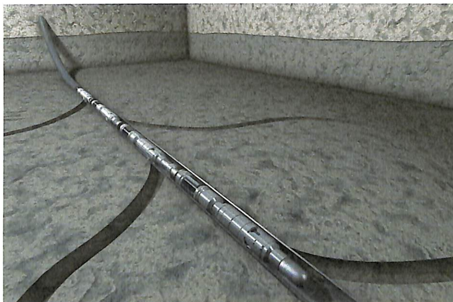
Figure 44 : Illustration of the Intelligent Completion inside the mainbore of a multilateral well to isolate and control inflow from each lateral
