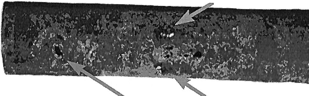
**Fig.4 bare pipe -not under cathodic protection**
