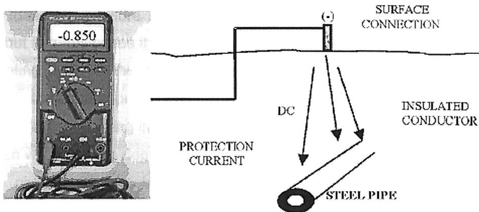
**Fig.9 Criterion 1 for cathodic protection**
