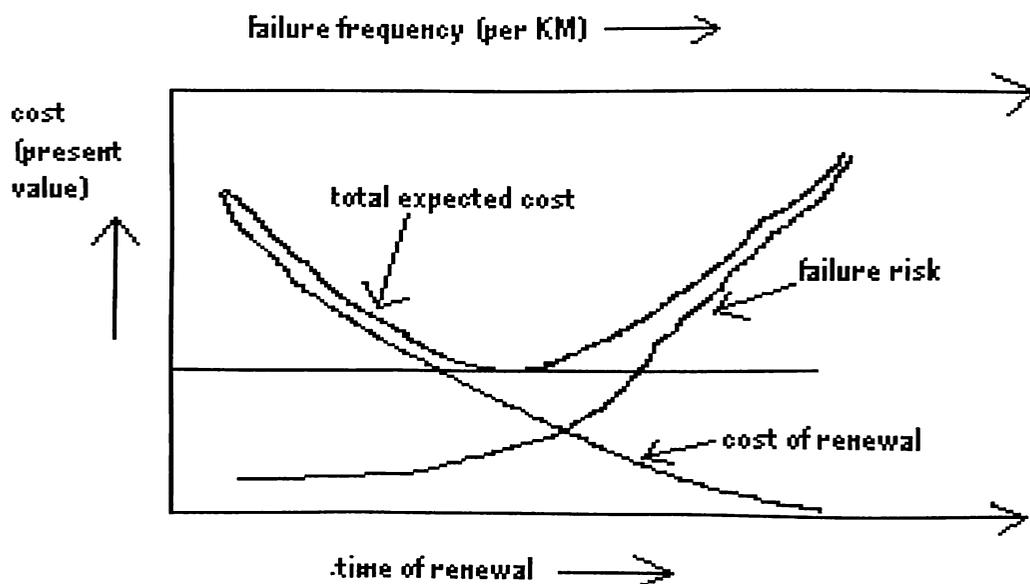
**Fig. 10 Deciding when to renew a pipeline with a high cost of failure.**
