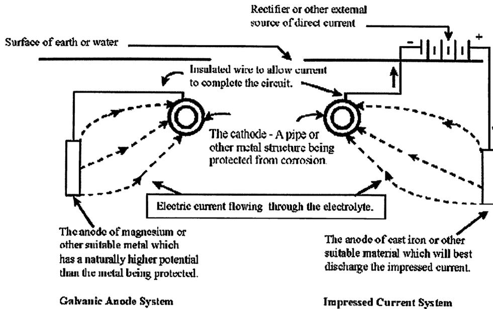
Fig. 8 Galvanic Anode System
