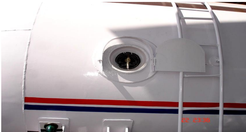
Figure 8 - Hydro carbon tanker with rotogauge
