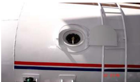
HYDRO CARBON TANKER WITH ROTOGAUGE
