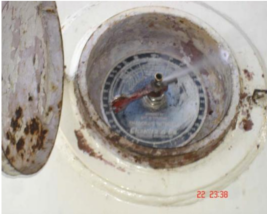
Figure 14– Opening of rotogauge to check liquid level inside the tanker
