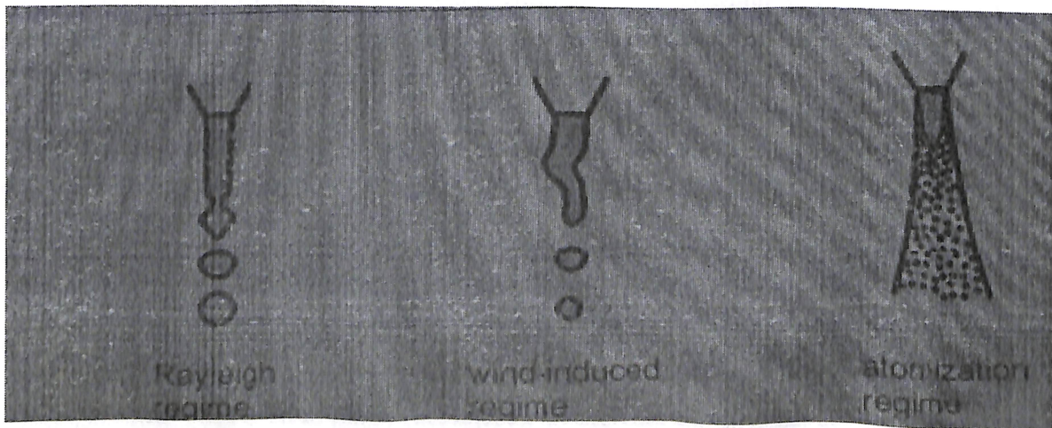
Fig. 2.1.1 (iii) Schematic description of jet break-up regimes
