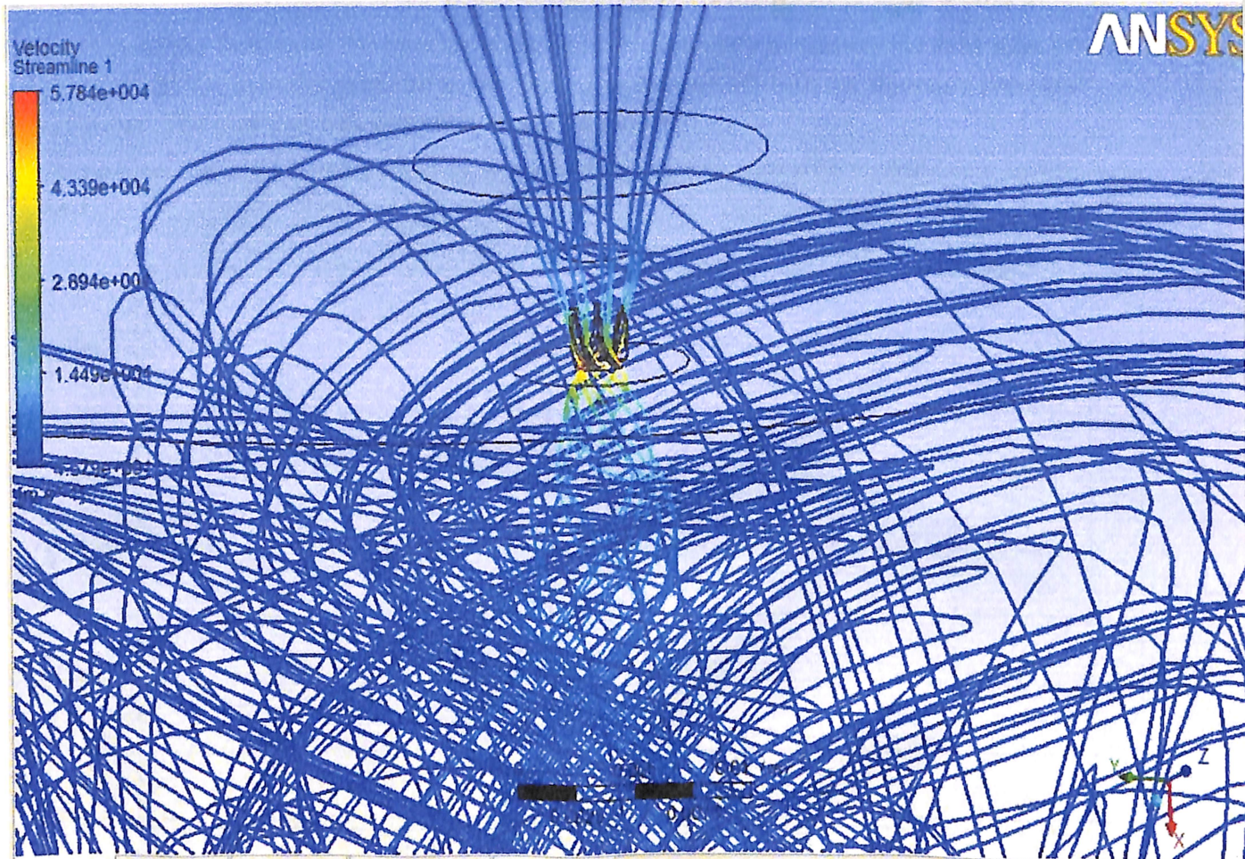
Fig.3.4 Injection Flow inside the cylinder volume
