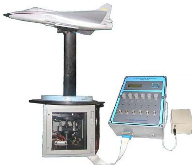
Figure 3.17: 6-Component Balance system used in the wind tunnel [148]
