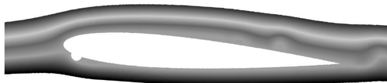
Figure 4.45: Roll up vortices for the protrusion height 0.02c located on the pressure surface, at 4^\circ
