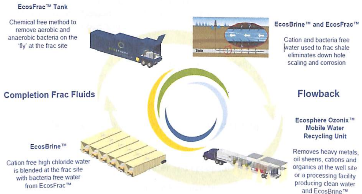
Figure 14.1: Total frac water management system
