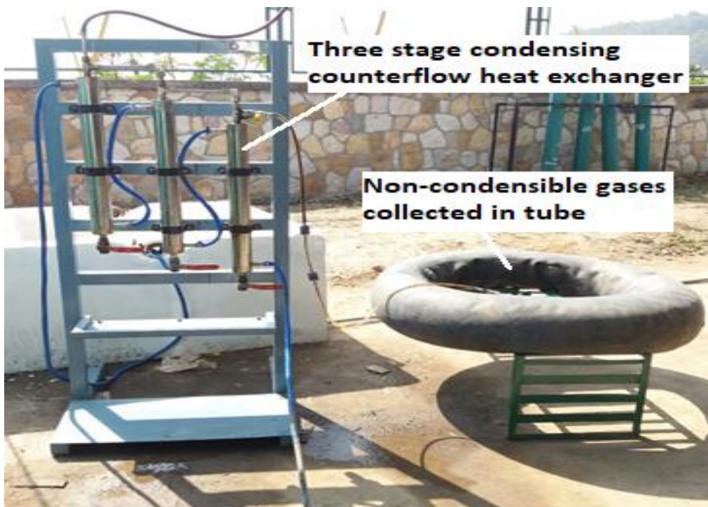
Fig 17: Photographic views of condensable and non-condensable gas collection
