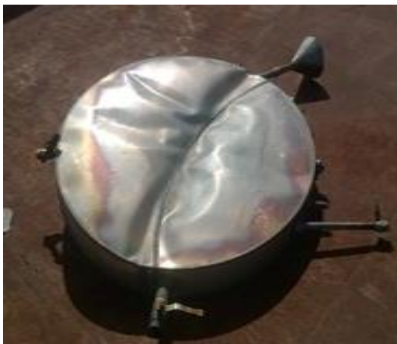
Fig. 11.3: Photographic view of Solar thermal pyrolysis reactor
