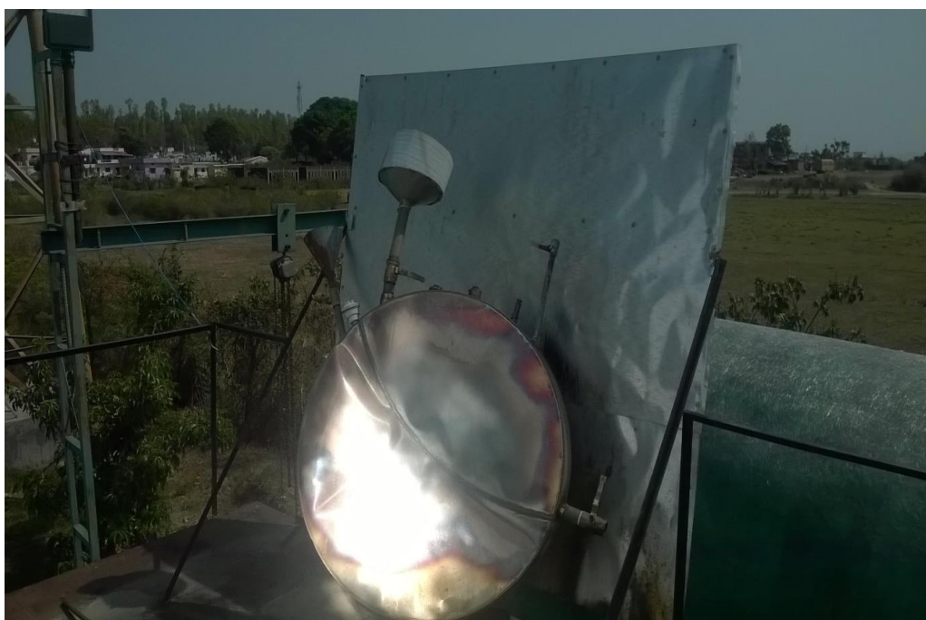
Fig. 11.2: Focused reactor place in front of Scheffler dish
