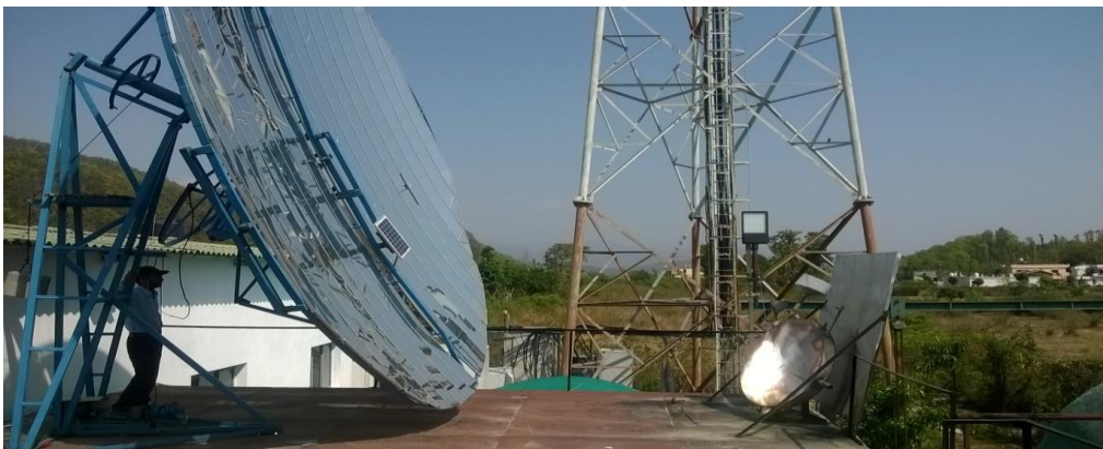
Fig. 11.1: Overall set-up for Solar Thermal Pyrolysis
