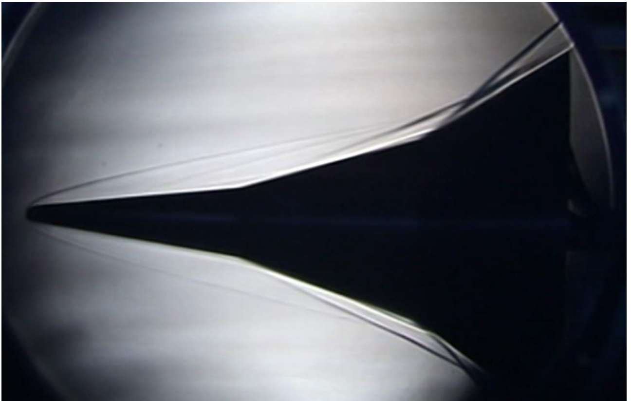
Fig. 7.37. Schlieren Image of Flow over triple ramp with 15^\circ third ramp angle
