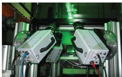
High Speed time resolved PIV System
