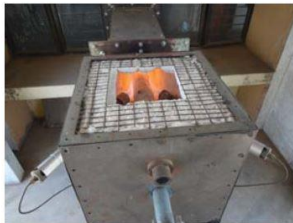
Fig. 7.8. Auxilliary Heating system (Courtesy: HSWTC Brochure)
