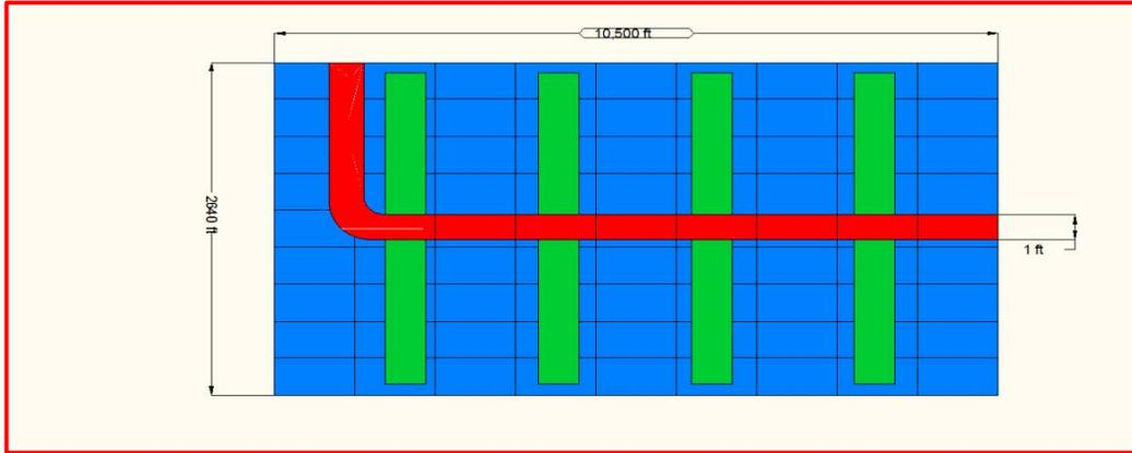
*Figure 4.4(d): Schematic Representation of a Four Hydraulically Fractured Reservoir.*
