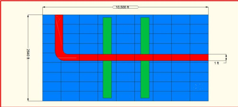
Figure 4.4(b): Schematic representation of a Two Hydraulically Fractured Reservoir.
