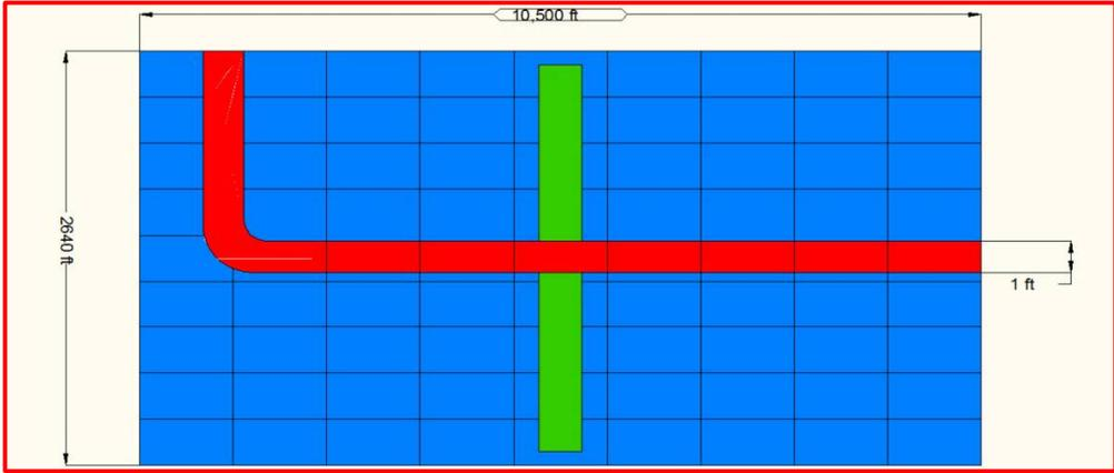
Figure 4.4(a): Schematic representation of a Single Hydraulically Fractured Reservoir.
