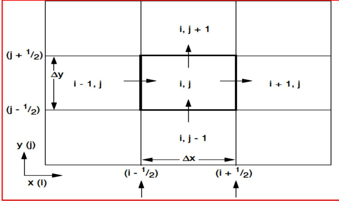
Figure 4.2: Discretization and notation indication for a 2D pressure equation for Matrix.
