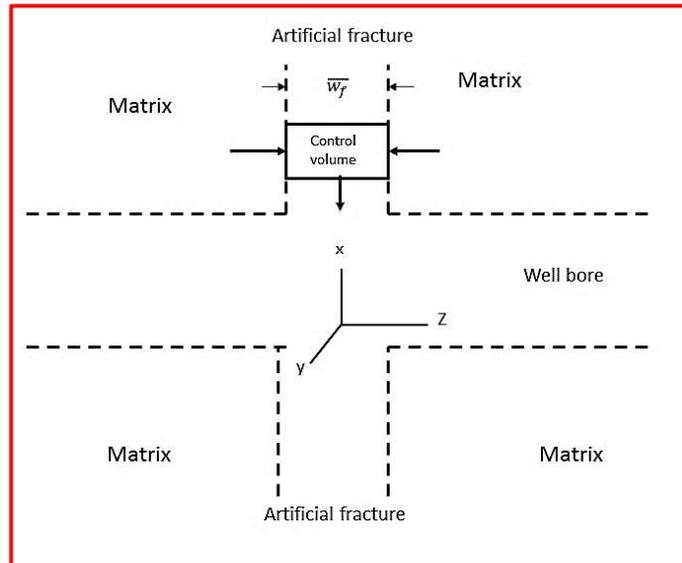
Figure 4.1: Schematic flow of gas in the hydraulic fracture.
