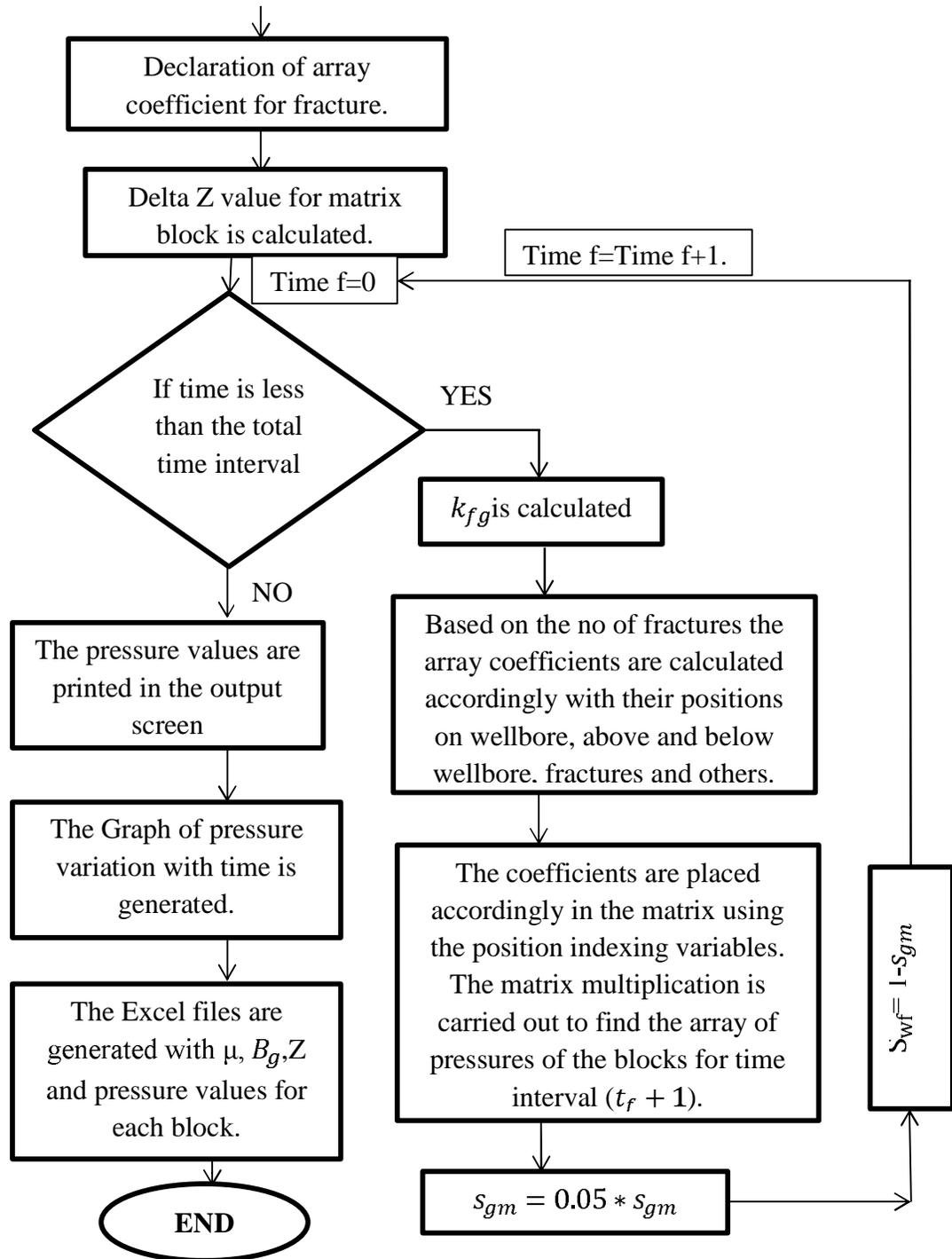
Figure 4.5: Algorithm representing the procedure for solving the gas flow in the hydraulic fractures.
