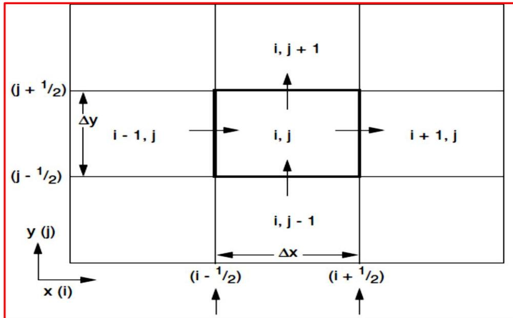
Figure 4.3: Discretization and notation indication for a 2D pressure equation for Hydraulic Fracture.
