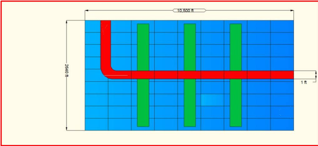
Figure 4.3(c): Schematic Representation of a Three Hydraulically Fractured Reservoir.
