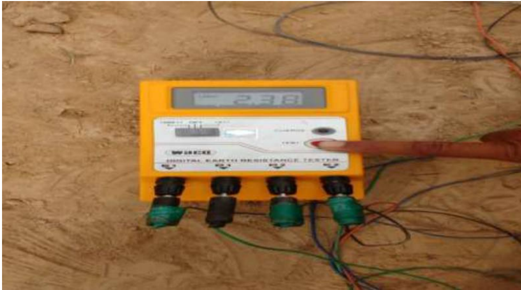
Fig 1.6 Resistance value shown by Earth Tester (WACO-MAKE)
