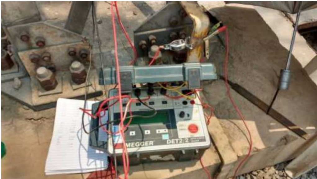
Fig 1.7 Resistance value shown by Earth Tester (MEGGAR-MAKE)
