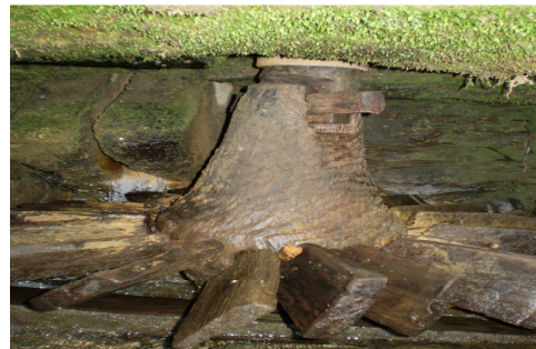
Fig 3.3: Traditional runner of a watermill at Ukhimath dated 23.06.2008 )
