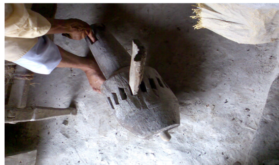
(Fig 3.4: Miller showing his damaged runner of a watermill at Ukhimath dated 23.06.2008 )
