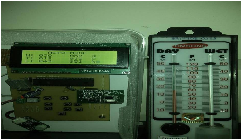
Fig.4.3 Snapshot for the testing of temperature sensor with standard thermometer
