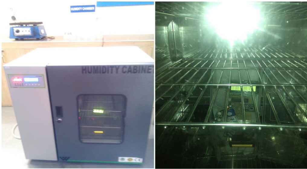
Fig.4.4 Snapshot for the testing of humidity sensor with standard instrument
