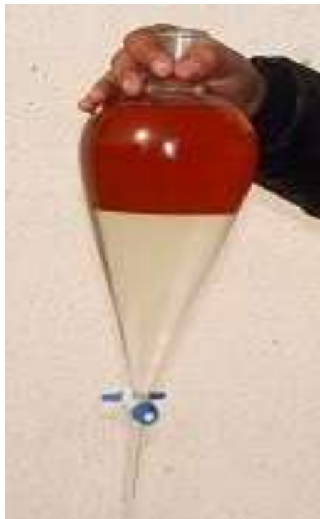
Figure 3.6: Biodiesel after trans-esterification and washing
