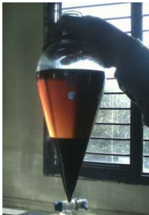
Figure 3.5: Feed stock in two layers after pretreatment
