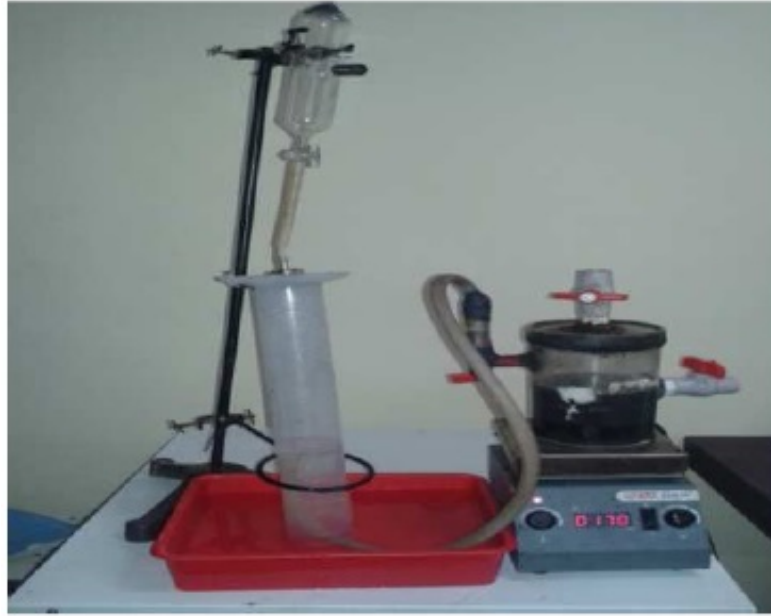
Figure 3.3: Anaerobic digester of 2 L capacity with water displacement method
