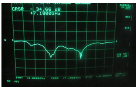
Figure 4.7: Return loss pattern of Third Test Antenna on the Display of VNA
