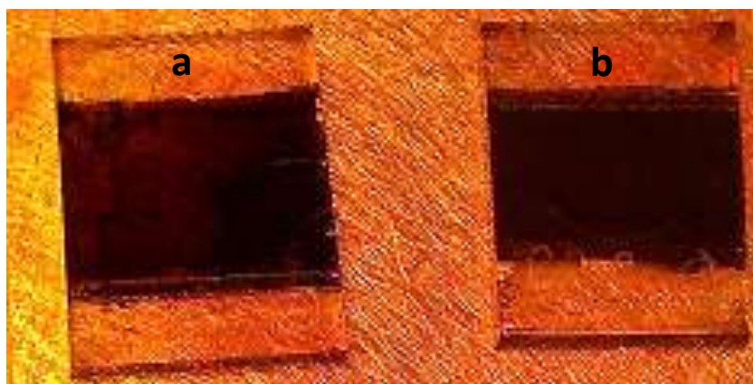
Figure 6.9: Pictures of perovskite films (a) PA-1/CH 3 NH 3 PbI 3 and (b) PA-2/CH 3 NH 3 PbI 3 .
