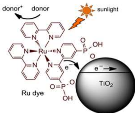
Figure 2.65: Schematic diagram showing the Ru dye anchored to \text{TiO}_2 nanoparticle.
