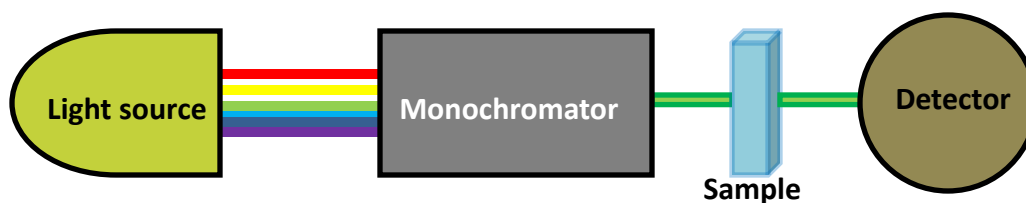
Figure 4.4: Key components of UV-Vis spectrophotometer.
