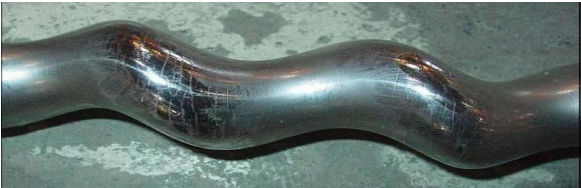
Figure 9 — Rotor cracked from excessive heat
