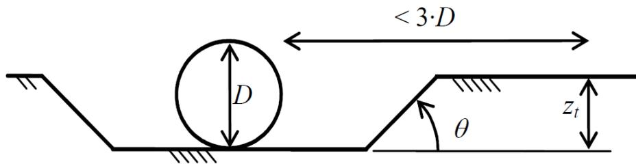
Fig 3.8: Definition of trench parameters
