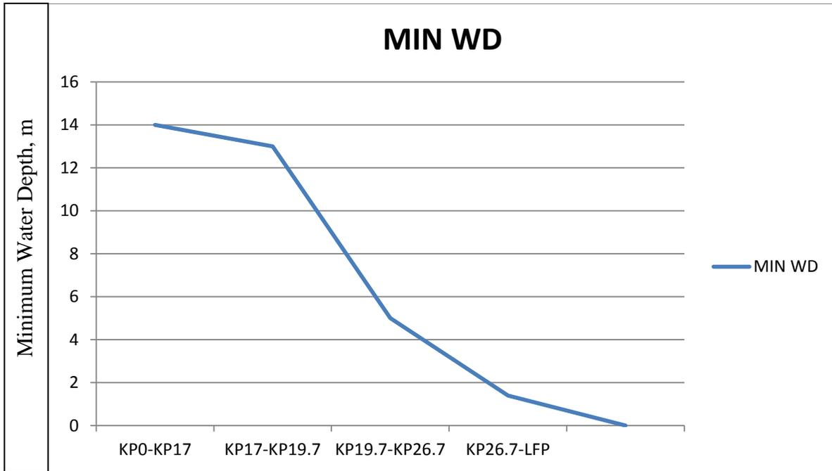
Fig 6.4: Minimum water depth along the pipeline route
