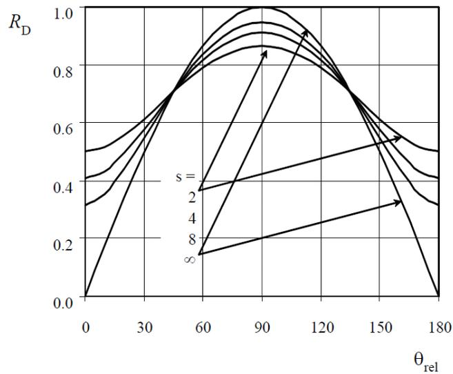
Fig 3.4:Reduction factor due to wave spreading and directionality
