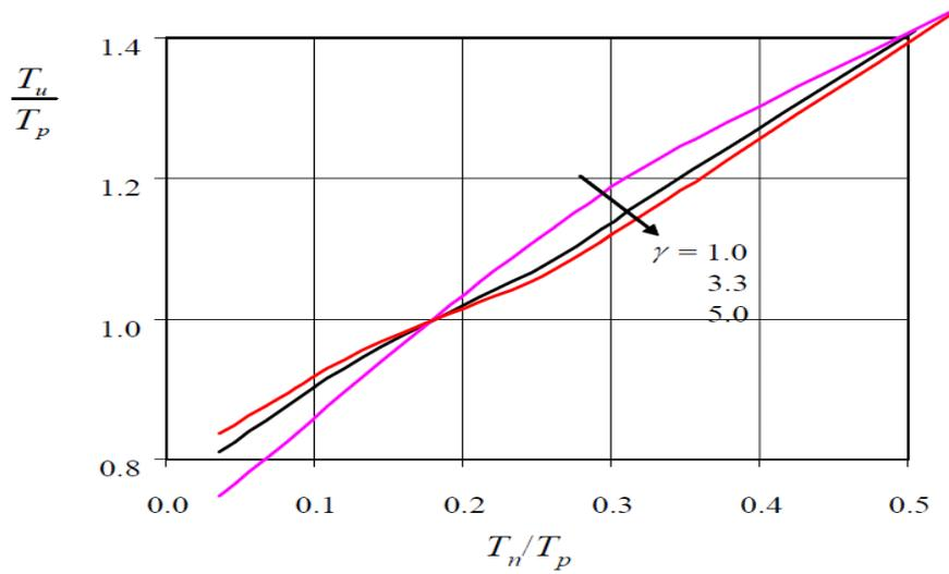
Fig 3.3: Mean zero up-crossing period of oscillating flow  $T_u$  at sea bed level
