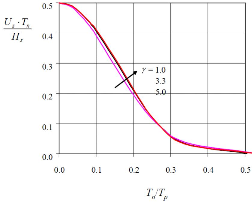
Fig 3.2: Significant flow velocity amplitude  $U_s$  at sea bed level
