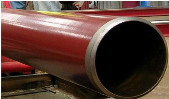
Fig 2.1 : Pipe with corrosion coating
