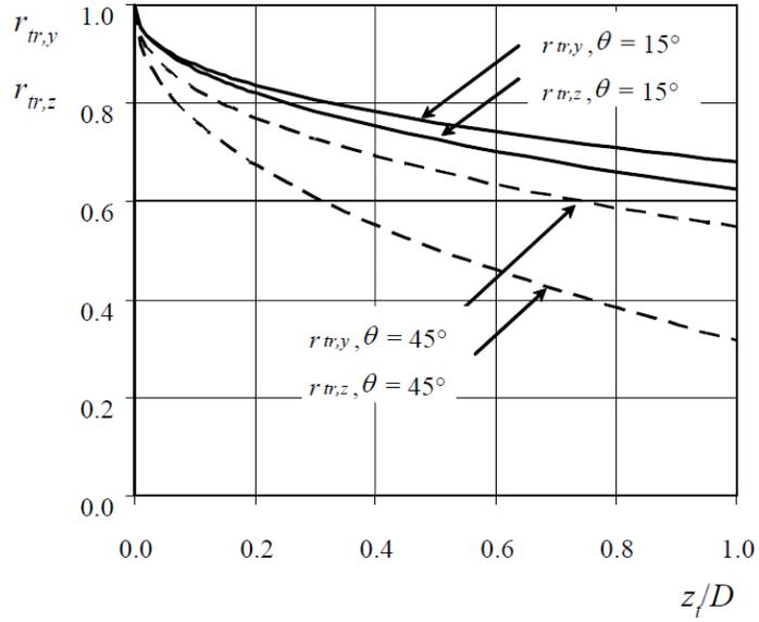
Fig 3.9: Peak load reduction due to trenching
