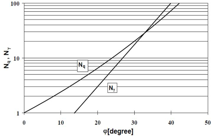
Fig: 3.1 Bearing capacity factors  $N_c$ ,  $N_q$ ,  $N_v$  versus the internal friction angle  $\phi_s$
