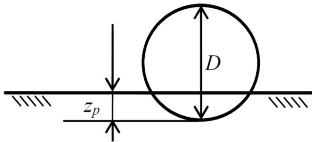
Fig 3.6: Definition of penetration
