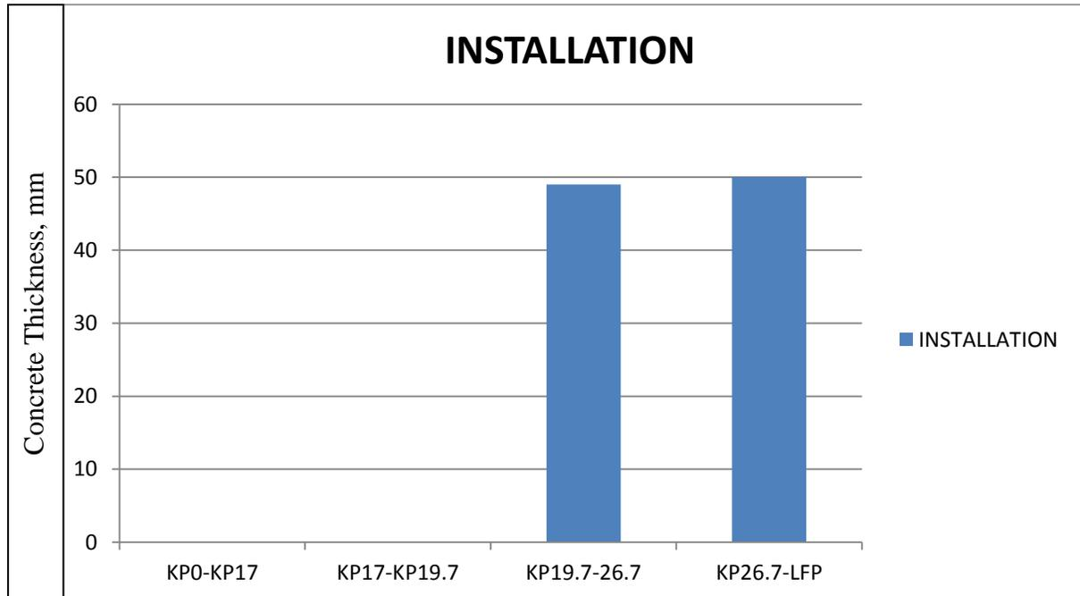
Fig 6.1: Required concrete thickness for installation condition
