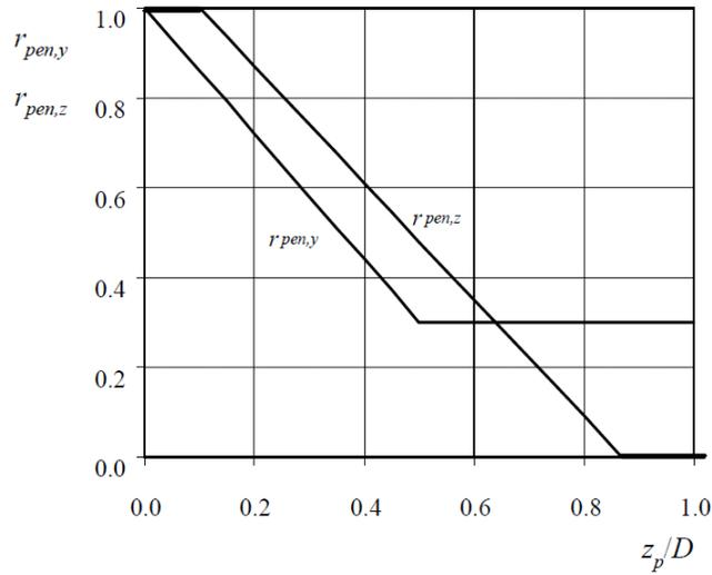
Fig 3.7: Peak load reduction due to penetration
