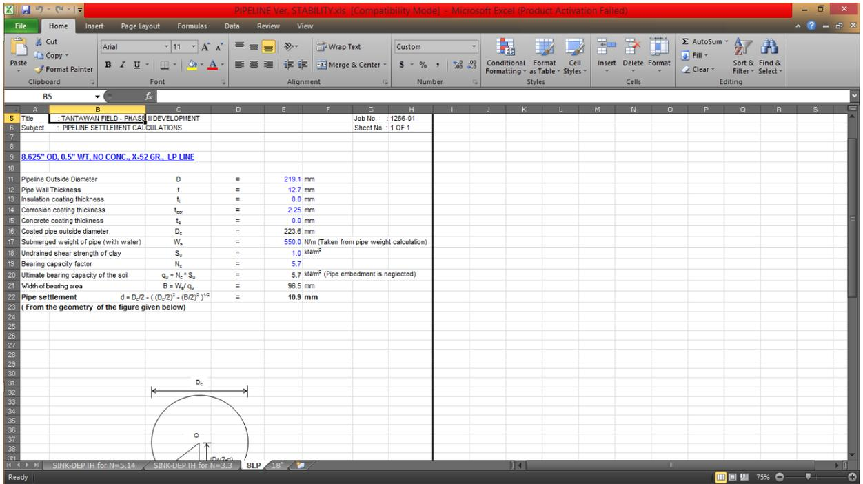
Fig 5.2 : Spread sheet (vertical penetration depth)
