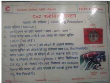
Fig 4.7: Description on CO 2 flooding system
