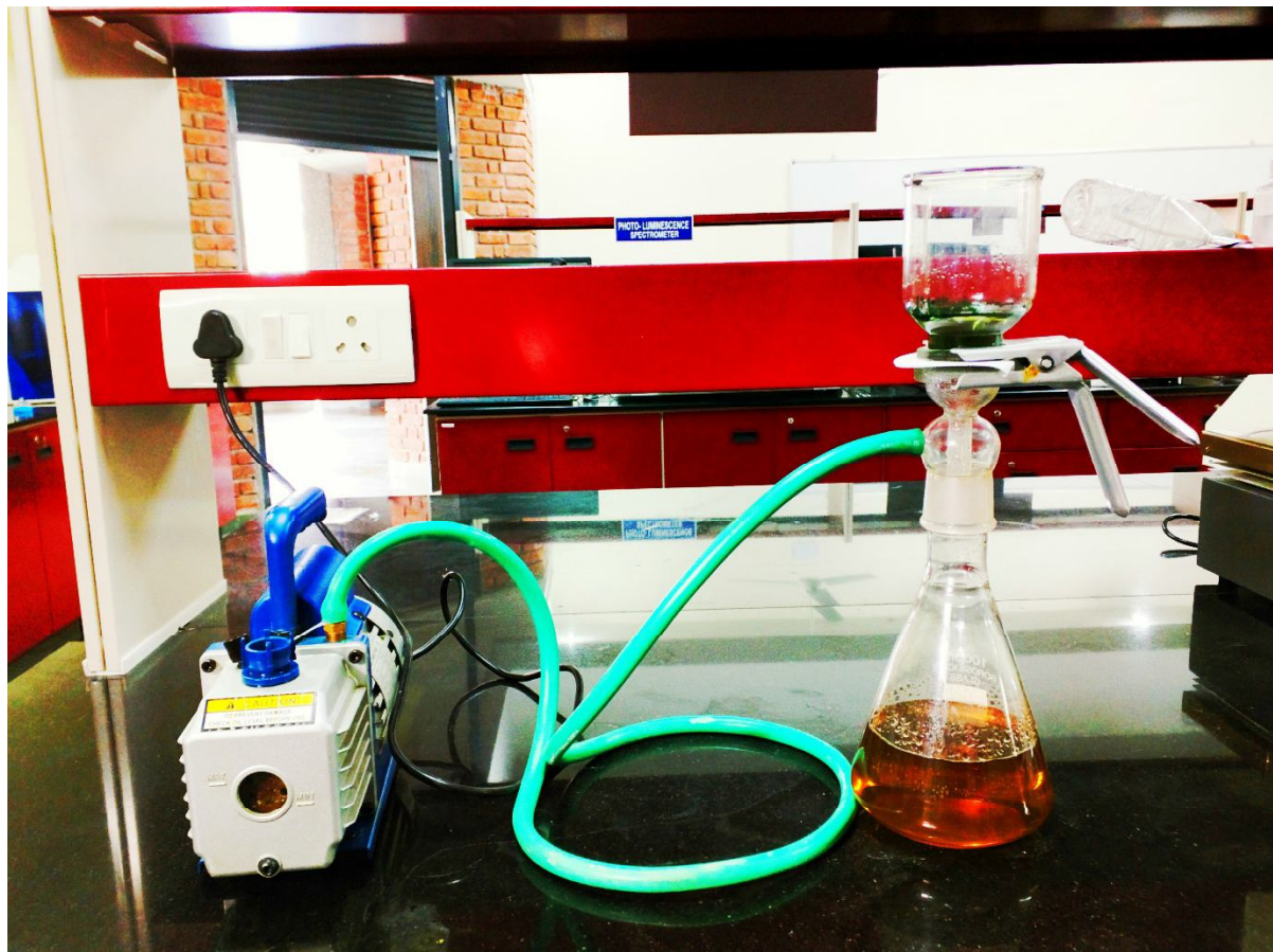
Fig. 2. Schematic of Vacuum Filtration of the samples
