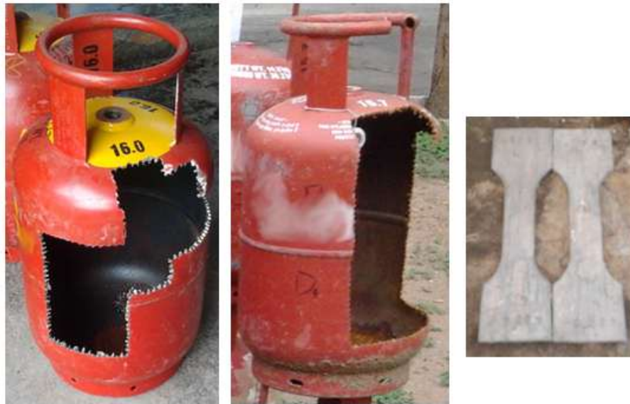
Figure 53: Example of two cut cylinders and a tensile specimen
