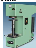
Fig.2: SAROJ Make Brinell's Hardness Testing Machine [13]
