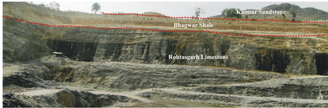
Fig. 2.11- Contacts of the Rohtasgarh Limestone, the Bhagwar Shale and the Kaimur Sandstone in Bistara Mine, Katni District, M.P.
