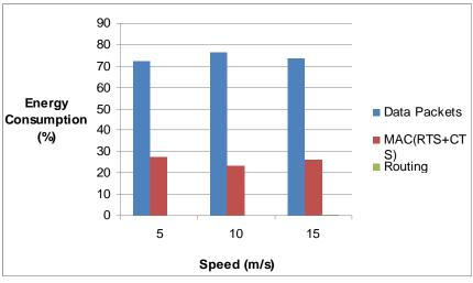
Fig. 4.8(b): Energy Consumption of DSR
