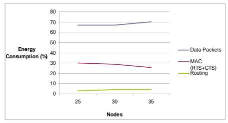
Fig. 4.7(a): Energy Consumption of AODV
