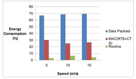
Fig. 4.7(b): Energy Consumption of AODV
