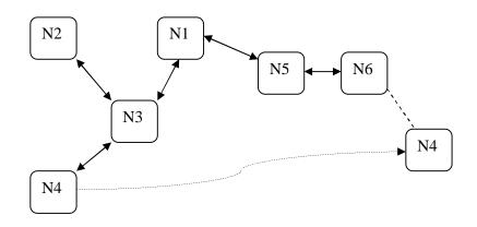
Fig 3.2: Example Network for DSDV
