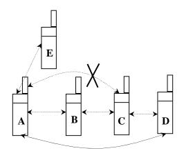
Fig. 3.1: An ad hoc wireless network
