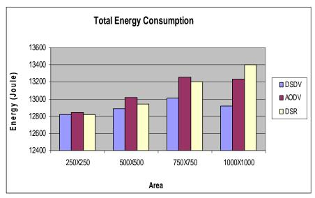
Fig. 4.4: Energy Consumption Vs Area
