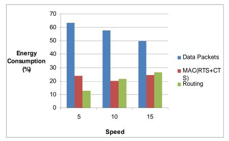
Fig. 4.9(b): Energy Consumption of DSDV
