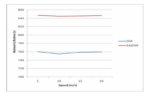
Fig. 6.4: Network Lifetime Vs speed
