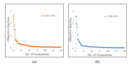
Figure 4.6: Improvement of the value of the objection function with generation number (a)  $(P_c, P_m) = (0.95, 0.02)$  (b)  $(P_c, P_m) = (0.98, 0.01)$
