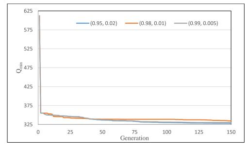
Figure 5.6: Variation of objective function ' $Q_{min}$ ' with generations for ( $P_c$ ,  $P_m$ ) = (0.95, 0.02), (0.98, 0.01) and (0.99, 0.005) for case (b)
