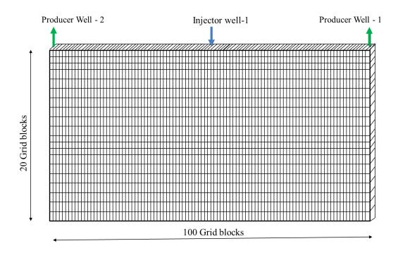
Figure 4.3: Schematic of synthetic reservoir
