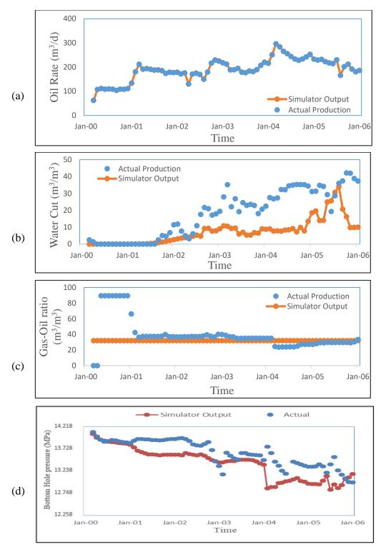
Figure 5.3 Case (a) - Comparison of simulator output of best initial ensemble (before optimization) with observed field values for (a) Oil rate (b) Water cut (c) GOR and (d) BHP
