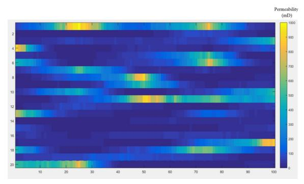
Figure 4.5: Initial permeability ensemble of 2-D synthetic reservoir
