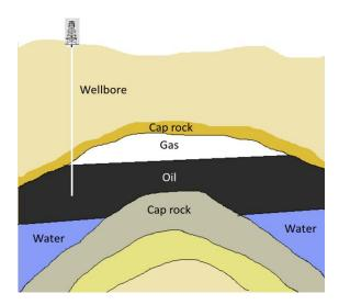
Figure 1.1: Schematic of a Hydrocarbon reservoir
