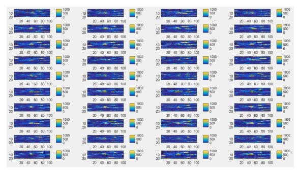
Figure 4.4: Initial permeability ensembles (40 Nos.) of the 2-D synthetic reservoir
