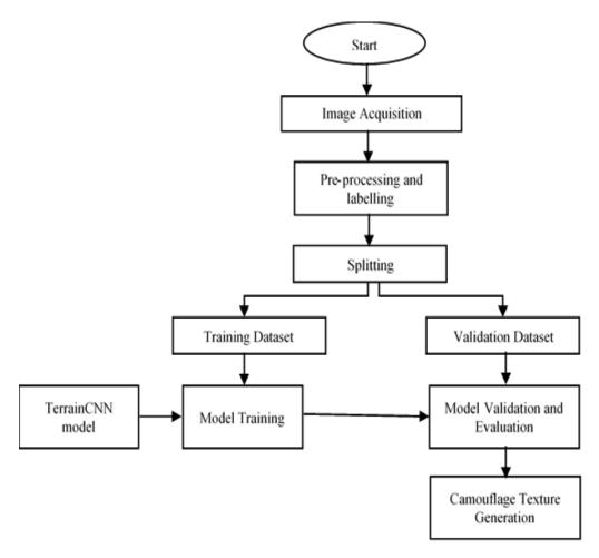
Figure 3-4: Terrain Classification using TerrainCNN
